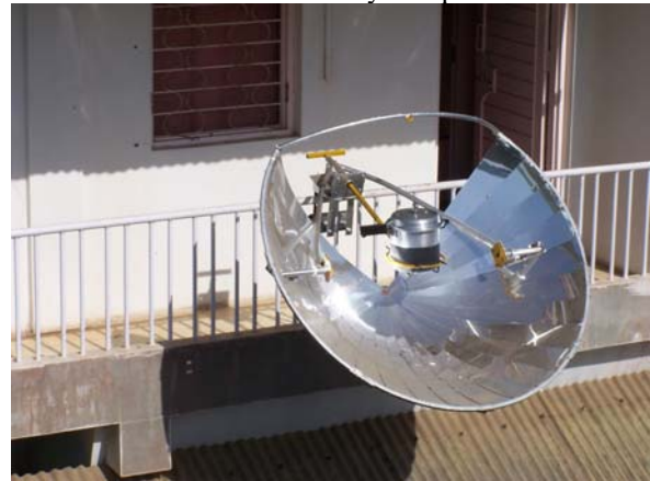
Photograph 1: Innovative balcony model of concentrating solar cooker:
