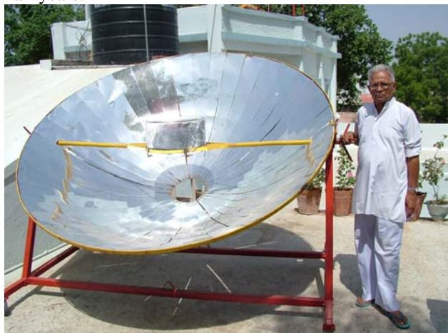
Photograph 1: Dr. P.T. Joshi with 2.3 m dia. parabolic dish concentrator, preparing ayurvedic syrups.
